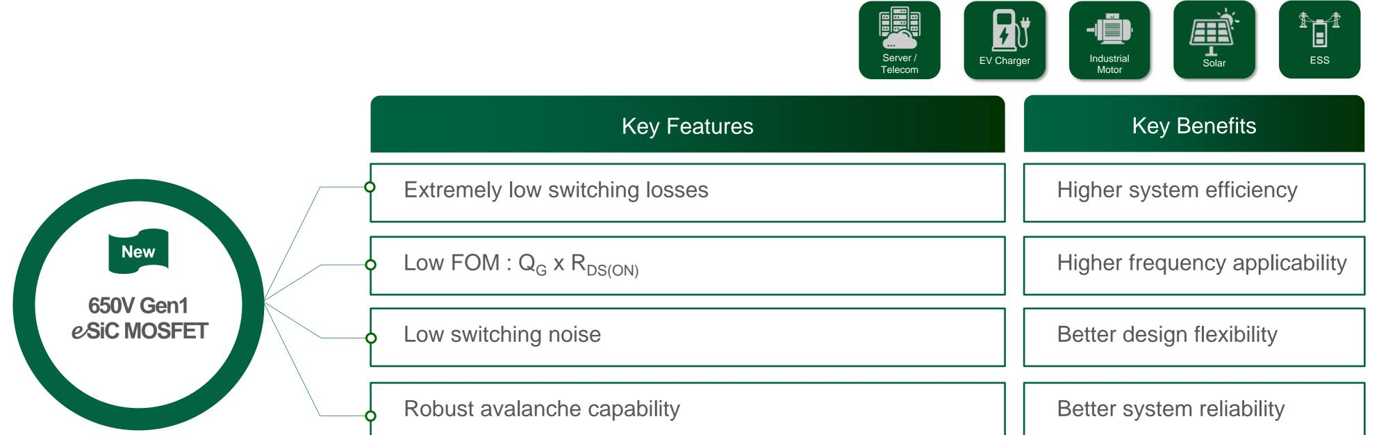
The 650V e/SiC MOSFETs enable innovative, high-performance PSU designs that reduce footprints while addressing thermal and electromagnetic interference challenges. These MOSFETs offer excellent switching performance, a stable threshold voltage for parallel operation, and 100% tested avalanche capability. They exhibit dramatically reduced switching losses, minimized voltage spikes, and lower dynamic C<sub>OSS</sub> loss, improving system efficiency and overall power savings.
